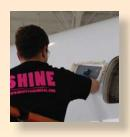
APPLY THE SHOULDER ZONE METHOD\* Beginning top right or left of target polish area, work back & forth, right to left. Then work same area up & down.
